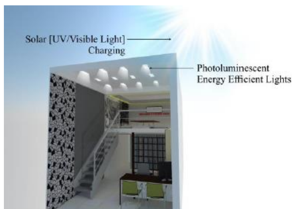
Figure 3. Proposed operational energy efficient lights in a corporate office.
